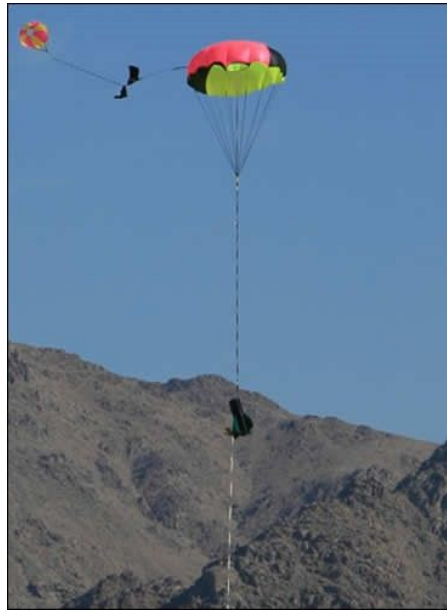
Figure 2: Dual deployment parachute system as it nears touchdown.
