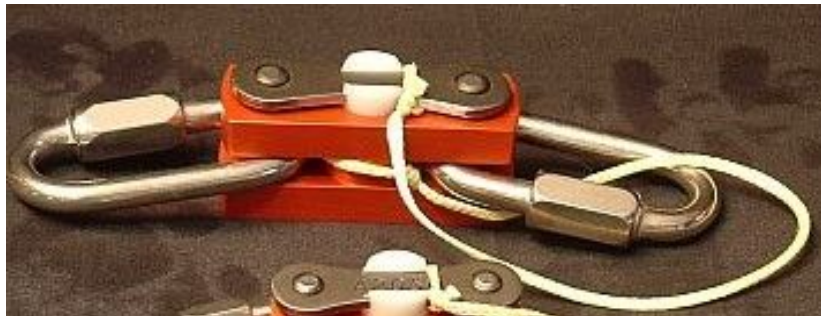
Figure 5: Quick release in the form of the tender Descender
